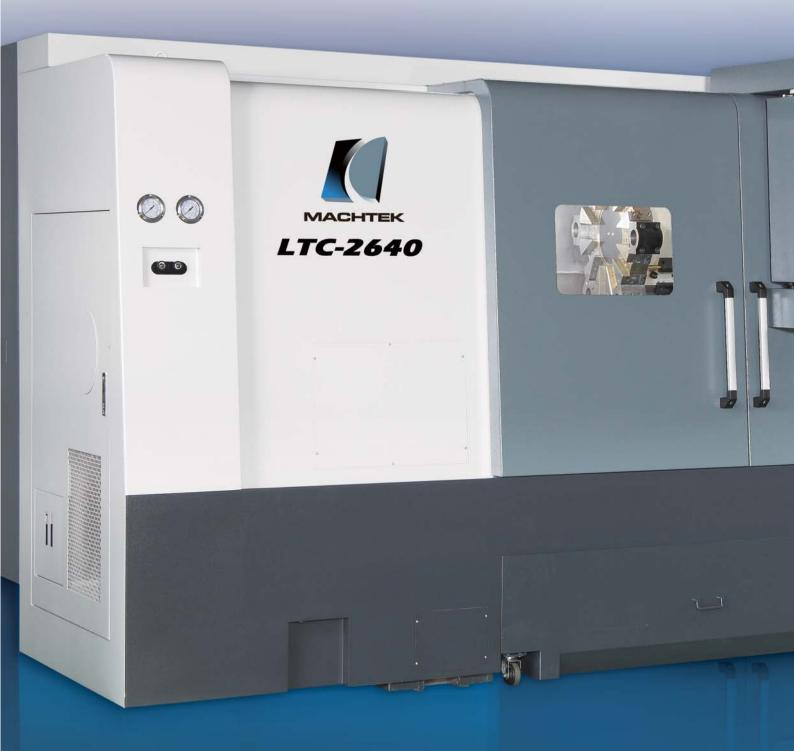
High quality fine grained cast iron base which incorporates a 45°slant bed design enhances stability to absorb cutting conditions of heavy workpieces. Guarantees the overall machine vibration dampening and long term accuracy.
