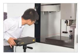
Every machine has been statically and dynamical inspection and compensated by laser measuring instrument.
