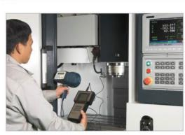
The IRD dynamic balancing device calibrates the spindle displacement, speed, and acceleration of the full speed range.
