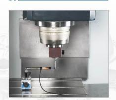
The Renishaw ball bar instrument calibrates the circularity and the geometrical accuracy to ensure the three dimensional motions precise.
